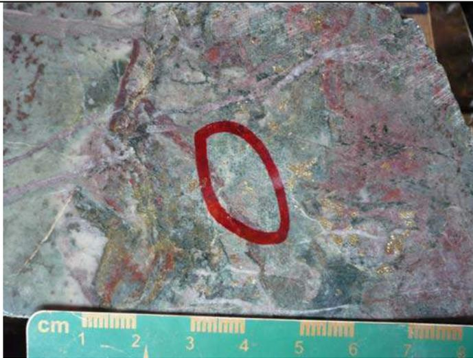
Photo 3: CP08-13 (86.9m; 10.34 g/t Au, 1.0 g/t Ag, 397 ppm Cu, 37 ppm Zn). Prograde garnet-diopside(?) skarn with irregular chloritization, PY-CP patches, visible gold.
