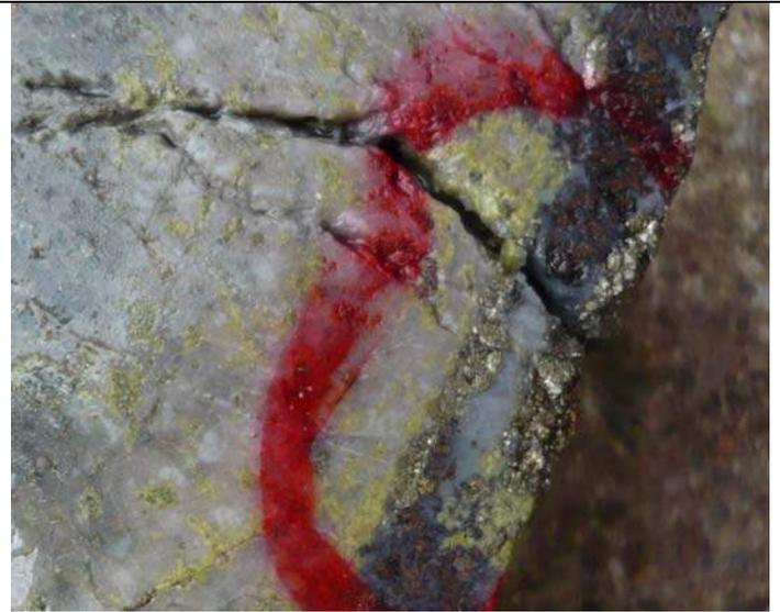
Photo 6: CA08-16 (115.0m; 10.93 g/t Au, 1.0 g/t Ag, 46 ppm Cu, 1073 ppm Zn). 5mm quartz-sphalerite-pyrite-gold veinlet cutting strongly sericitized feldspar(-biotite?) porphyry. Epidote along fractures.
