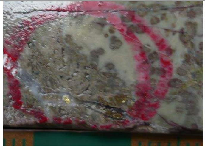
Photo 4: CP08-15 (51.3m; 3.40 g/t Au, 2.0 g/t Ag, 325 ppm Cu, 81 ppm Zn). Gold flake in centre of late anhydrite veinlet cutting pink garnet-diopside(?) skarn with 5% pyrite. Patchy chalcopyrite.
