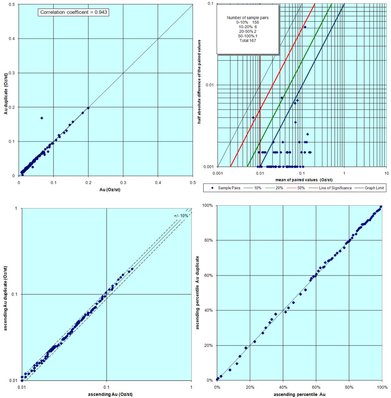
Note a) Normal Scatter Plot; b) Precision Pair Plot; c) log Q-Q plot; d) P-P plot
