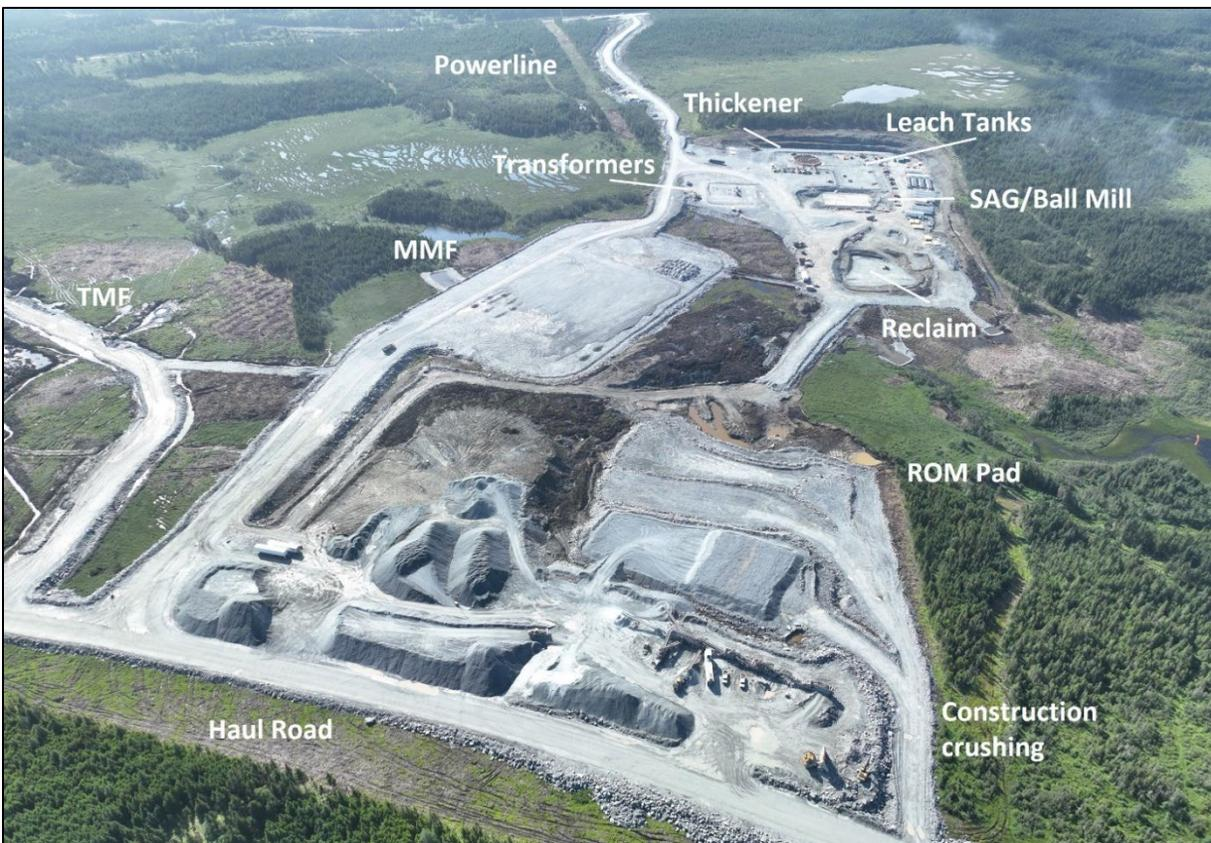
Figure 1: Valentine Process Plant Site, Looking South, July 2023. TME: Tailings Management Facility, MMF: Mine Maintenance Facility
